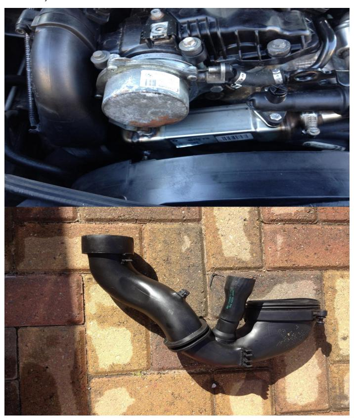
2. Now loosen the jubilee clip on the left side of the thermo housing and pull off the smaller pipe then unclip the hose also on the left side and gently ease it off (I gently persuaded mine with a large screw driver) once disconnected point the hose down to drain most of the systemcoolant out, use a drip tray, container or driveway. Then take your T40 torx bit and undo the 2 bolts that secure the EGR cooler back to the engine (top left hidden away on the pic below)
