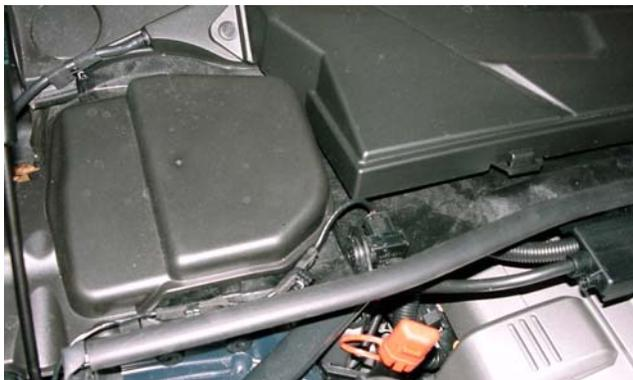
**E-box Cover, AUCII Sensor, and Microfilter Housing**
