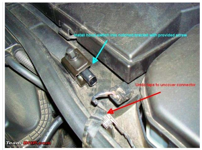
Remove plug from connector and insert the connector into hood-switch. It'll only go in one way.
