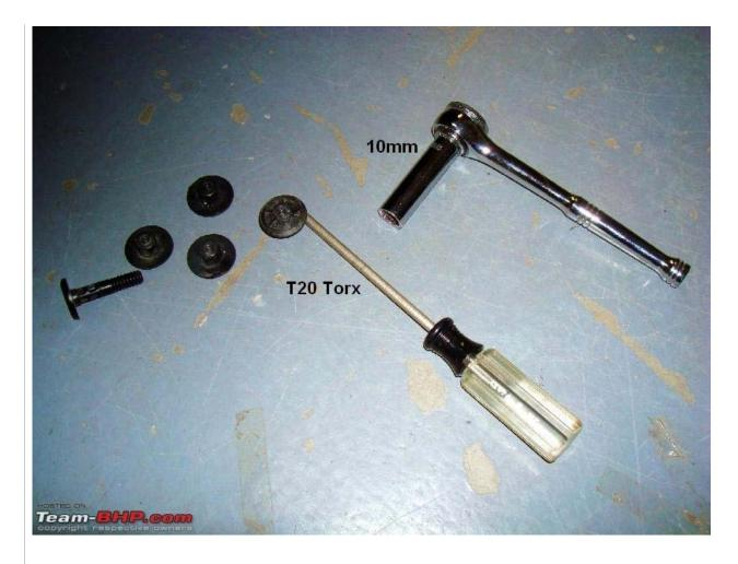
After removing the 4 bolts and the torx screw, peel back the wheel liner over the brake and leave it there.
