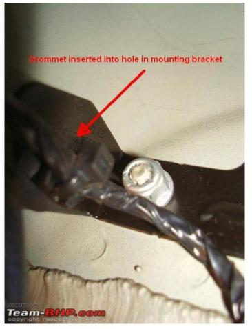
Plug the hanging connector into the slot on the siren - it'll only go in one way. Fasten the mounted siren plate, to the mounting bracket using the remaining 2 hex-head screws. (Make sure that wires aren't pinched between the bracket and the mounting plate).
