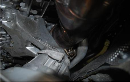
4. Unbolt both O2 sensors that are located after the turbo. See (Fig.1)
