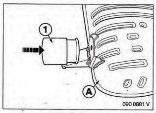
Uninstall acoustic distributor (1) on the standard silencer (not shown) and fit it to Performance silencer **A**.
