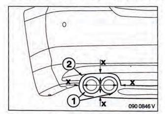
Check the position of the end pipes (1) to the contour (2) of the rear apron, if necessary averaging and aligning them again. ◀
