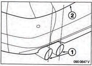
During installation and while driving (thermal expansion of the exhaust system), care must be taken to ensure that the end pipes (1) do not extend beyond the rear apron (2). (Danger of burning!) ◀
