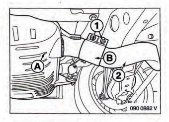
In order to ensure adequate ground clearance, the screws (1) must not be below the pipe geometry and must be directed appropriately upwards, as shown in the figure. The screws (1) must have a distance of **20 mm** to all neighbouring components.
