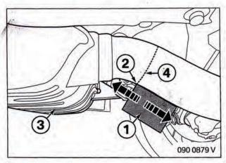
Using a suitable flat object (1), determine and mark (4) the start of the curve (2) of the entrance pipe into the rear silencer (3) by moving the flat object (1).
