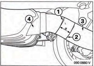
From the marking (1), draw a mark (2) at a distance of **a = 40 mm** on the entrance pipe (3).
