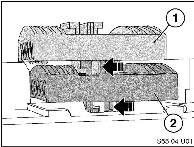
8. Separate upper black junction block (1) from lower black junction block (2) by pushing locking tab (black arrow) to the left and sliding upper block rearward.
