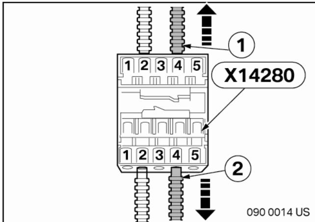
**Warning:** Label all fiber optic cables removed and/or relocated during this installation including position location and orientation (input vs. output) to avoid MOST ring errors.
