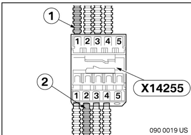
14. Connect the SDARS fiber optic cable (1) removed from junction block X14280 in Step 11 into the empty slot **Position 1** of junction block **X14255**.
