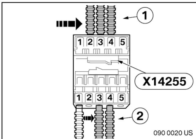
**Note:** The number of fiber cables connected to MOST junction block X14255 may differ than shown, depending on vehicle options.
