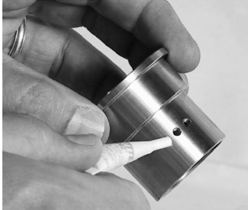
9. Lube up the UUC EVO shifter. Follow their instructions and liberally grease the upper and lower plastic bushings, pivot ball etc.
