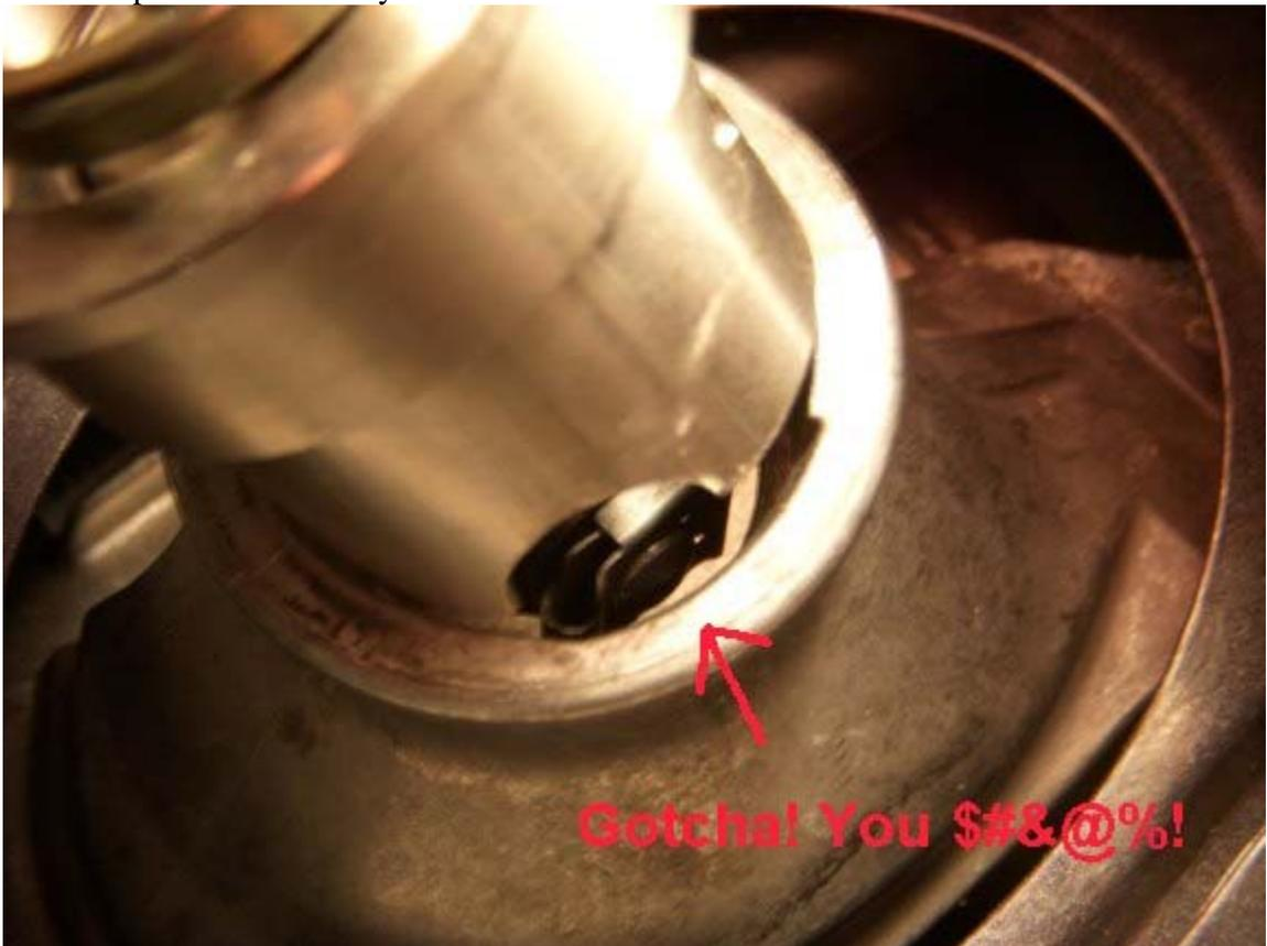
13. Push rags or paper around the shifter carrier so if you drop a screw it can't fall into the 'pit of no return' (trans heat shield- don't ask how I know this).
