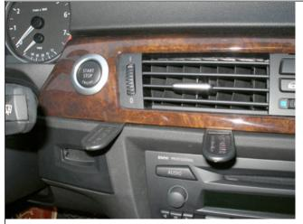
1. Press the thin end of the enclosed gap openers upwards into the gap between the wood grain trim and the climate control panel frame, to widen the gap. Peel off the cover of adhesive tape on the ProClip.
