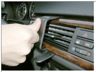
3. Press forward on the upper part of the ProClip so the angled edge snaps over the wood grain trim and into the gap between the trim and the padded part of the dashboard. Press until you see or hear/feel it snaps into place. Pull out the gap openers
