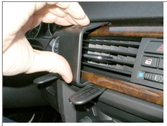
2. Place/hook the grooved edge on the lower part of the ProClip into the gap between the gap openers.
