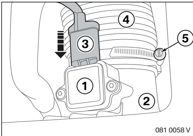
Connect the mass airflow meter (1) to intake filter housing (2) using plug (2).
