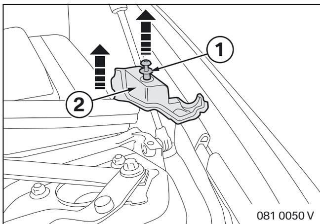
Remove the plastic expanding rivet (1) and adapter (2).
