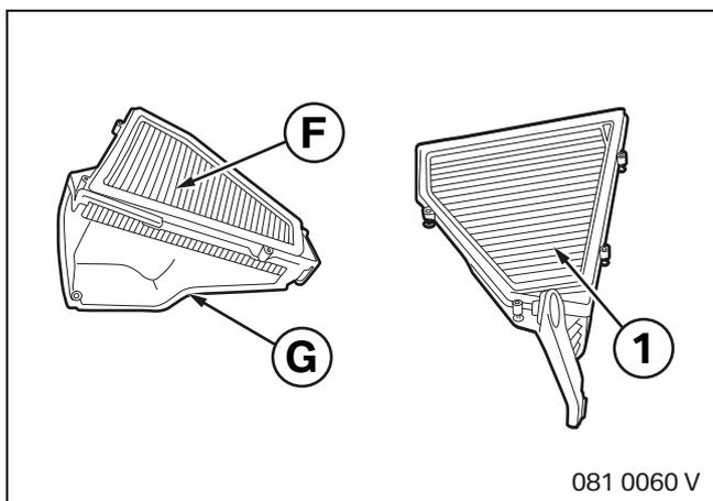
Place the Sport air filter insert **F** in the new front section of the intake filter housing **G** and connect to the old rear section of the intake filter housing (1).
