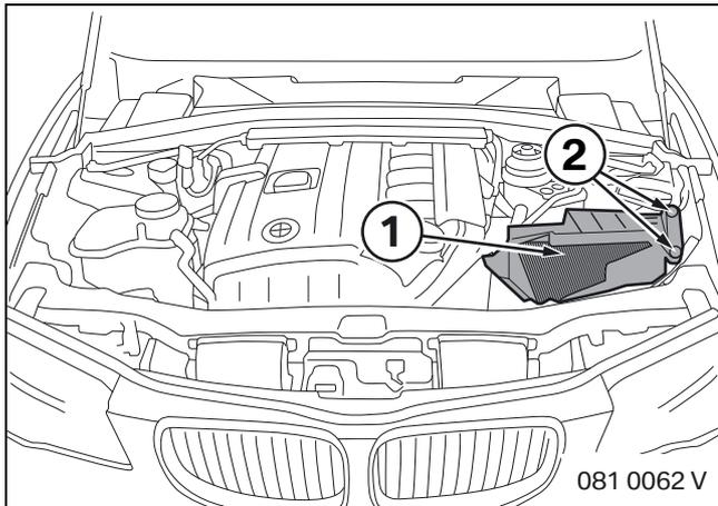
Place the intake filter housing (1) in the engine compartment and secure in place with screws (2) from the removal process (ISTA no. 13 71 000).
