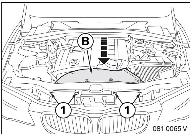
Connect the carbon intake channel **B** to the front.
