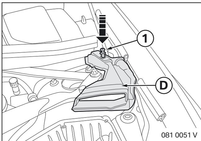
Secure the air guide **D** using the plastic expanding rivet (1).
