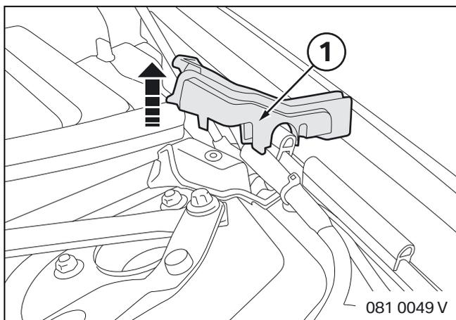
Pull the bonnet seal (1) upwards (clipped).
