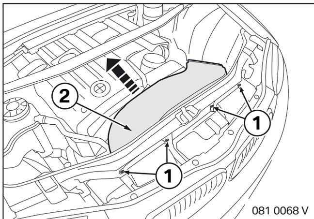
Unscrew the Torx screws (1) on both sides.
