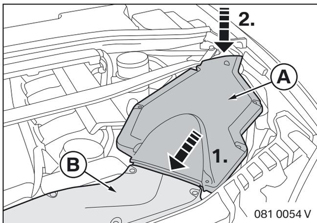
Introduce the upper section of the intake filter housing **A** into carbon intake channel **B** and then place it on top of the intake filter housing.
