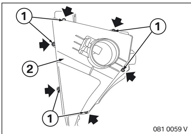
Undo the Torx screws (1) on the intake filter housing (2).
