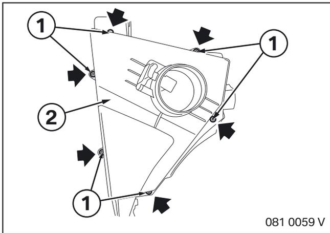
Use the existing Torx screws (1) and reassemble the intake filter housing (2).
