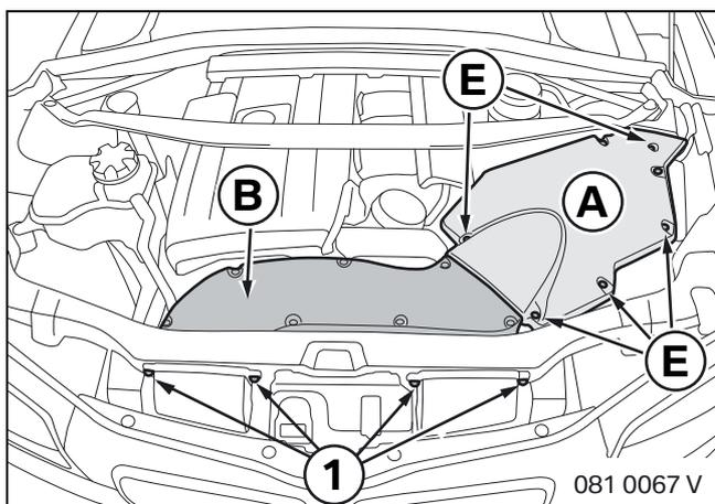
Secure the upper section of the intake filter housing **A** in place using the supplied screws **E**.
