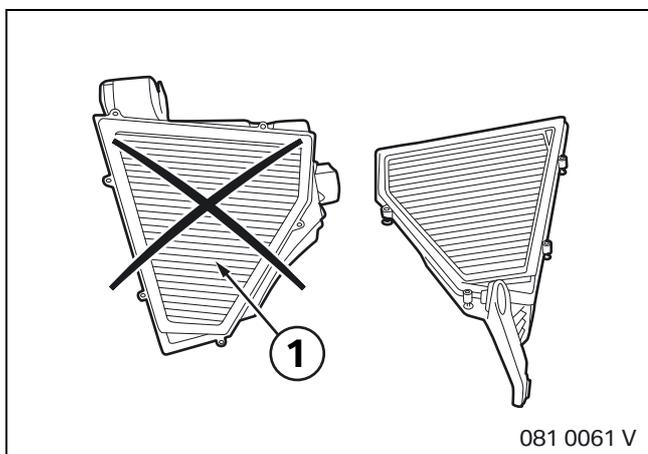
Dismantle the air filter housing and remove the front part, including the standard air filter (1).
