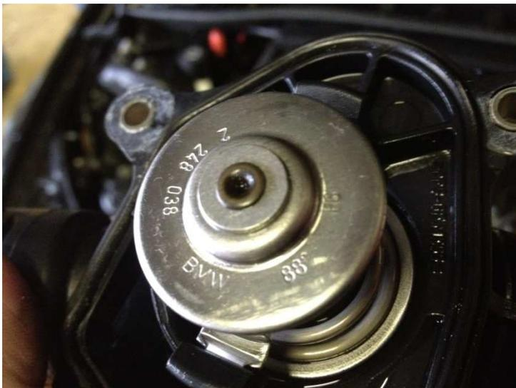
Install new thermostat taking care not to undo the seal...also oil up the bolts that hold stat in place as they can be dry.
