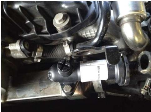
You now must remove the stainless steel pipe coming from the EGR heat exchanger to the EGR itself. Using a 7mm socket undo both jubilees at either end and take out this pipe. Note the jubilees have clamps inside and you may need to also pry open a bit with a screwdriver.
