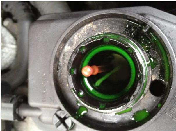
I took the car on a half hour road test and when I started the coolant temperature was 78degC. It steadily rose to 91 degC within 5 min and found a happy medium of 91-93degC, this was driving moderately at 50mph in steady traffic with max rpm 2,000. The ambient was 8degC and the AC was on 20degC both sides. During the journey I carefully opened the expansion tank to let out any trapped air.
