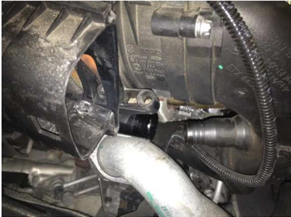
The EGR heat exchanger now must come out; you'll need an Allen socket and a torx on the exhaust end. Undo both Allen bolts that are closest to where EGR stat was, then undo other Allen bolt on left (NOTE ITS THE LONGER BOLT DO NOT REPLACE IT IN THE WRONG SIDE OR YOU MAY DRIVE IT INTO THE TIMING CHAIN)
