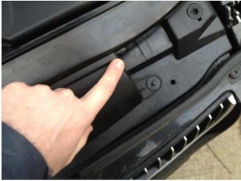
Now you can start undoing the EGR 'stat. Note it's clean and still has the part no. Attached (a few weeks old)! For this take a 7 & 10mm socket and torx head. Open the jubilee and pull the hose off (tie out of the way to preserve coolant). Undo the oil breather and pull it well out of your way. You can now access both 10mm nuts holding in the EGR stat...Undo those and lift out the stat.
