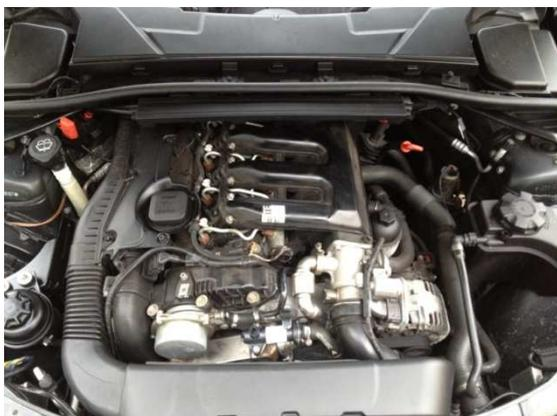
Undo the air intake duct above the kidney grille, there are two torx screws left and right and one on top, then using a flathead take out the flexible hose the connects onto the intake silencer.
