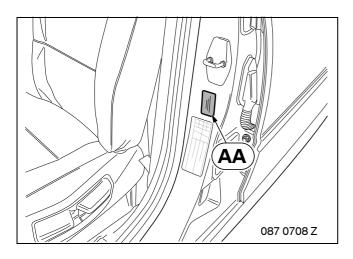
Apply **AA** information plate in visible location on driver's side B-pillar.
