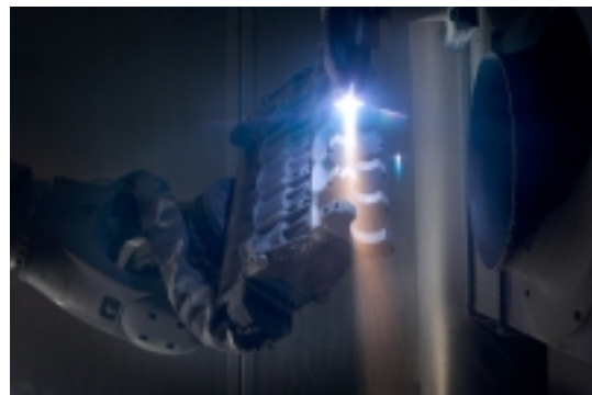
Figure 10: Arc spraying process
