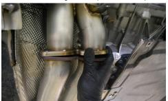
3. Next you will need to unbolt the V flange near the turbo. Keep the hardware as it will be reused (Fig.2)
