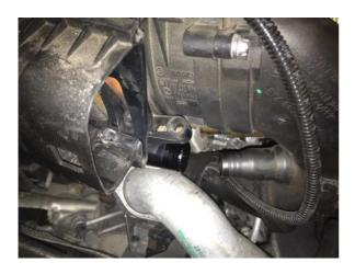
The EGR heat exchanger now must come out; you'll need an Allen socket and a torx on the exhaust end. Undo both Allen bolts that are closest to where EGR stat was, then undo other Allen bolt on left (NOTE ITS THE LONGER BOLT DO NOT REPLACE IT IN THE WRONG SIDE OR YOU MAY DRIVE IT INTO THE TIMING CHAIN)
