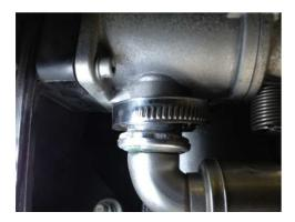
Now you need to remove the air intake from the other side of the cleaner element that connects onto the turbo (oddly enough has no clip) on top you need a T20 female torx and there is nothing on the bottom just pull the hose off the turbo. Take care with a small 3-4 inch pipe in the middle of the larger pipe (no clips just pulls off too)
