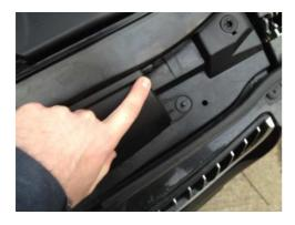
Now you can start undoing the EGR 'stat. Note it's clean and still has the part no. Attached (a few weeks old)! For this take a 7 & 10mm socket and torx head. Open the jubilee and pull the hose off (tie out of the way to preserve coolant). Undo the oil breather and pull it well out of your way. You can now access both 10mm nuts holding in the EGR stat...Undo those and lift out the stat.
