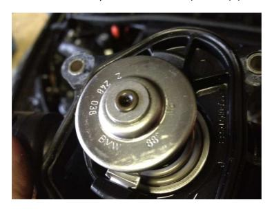
Install new thermostat taking care not to undo the seal...also oil up the bolts that hold stat in place as they can be dry.
