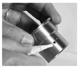
The objective is to take off only as much material as needed in the space between the two sets of (3) screw holes on the cup so when we tilt the cup you can see the selector rod and shifter mating point enough to slide on the retaining clip. This (installing retaining clip) is really easy to do with a stock shifter but with the UUC it is basically impossible.
