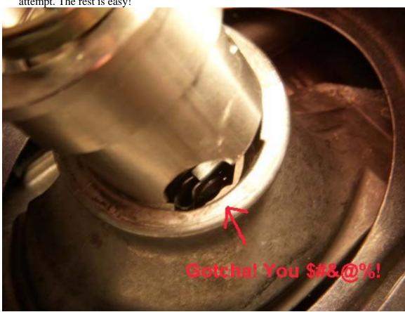
13. Push rags or paper around the shifter carrier so if you drop a screw it can't fall into the 'pit of no return' (trans heat shield-don't ask how I know this).
