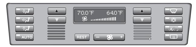
The control module contains a fault memory in a non volatile RAM and incorporates a sleep mode when the ignition is switched off. The control module will switch to the sleep mode 16 minutes after the ignition is switched off. The control panel consists of the following:
