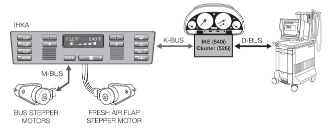
Replacement values are stored in the control module that will allow the IHKA system to continue to function when various sensors fail. Output faults result in the switching off of the failed output.
