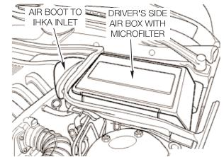
Care must be taken when servicing the micro filters or moving them for access to other components. When reinstalling the filters, ensure that the seals are properly installed to prevent odors from entering the interior.
