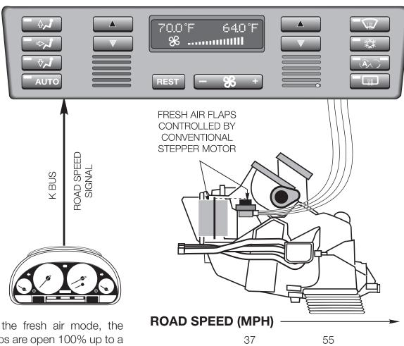
In the fresh air mode, the flaps are open 100% up to a road speed of approximately 37 MPH at which point they are closed to 40%.
