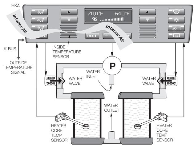
The auxiliary water pump is used to ensure that a sufficient volume of coolant is available to the heater cores for all heating conditions. The auxiliary pump is also used to supply coolant for the "REST" feature of the IHKA. The auxiliary water pump is powered directly from the IHKA control module through a final stage output.
