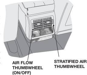
The stepper motor is operated by the control panel/module using information from the console rear outlet thumbwheels and the control panel/moduel buttons (left air distribution
