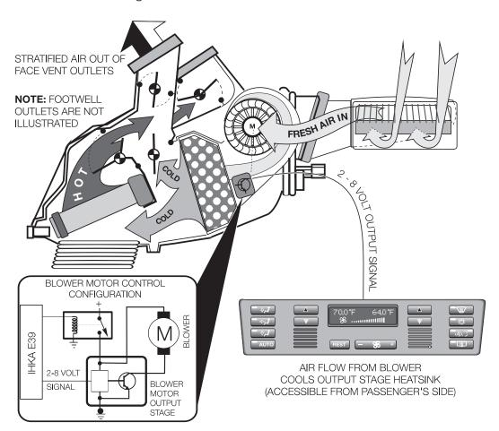
The blower motor is controlled through an output stage that is mounted in a heat sink on the heater case.
