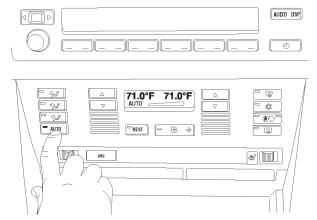
The operation and appearance of the IHKA on the E39 as of 9/96 production has changed only slightly:
