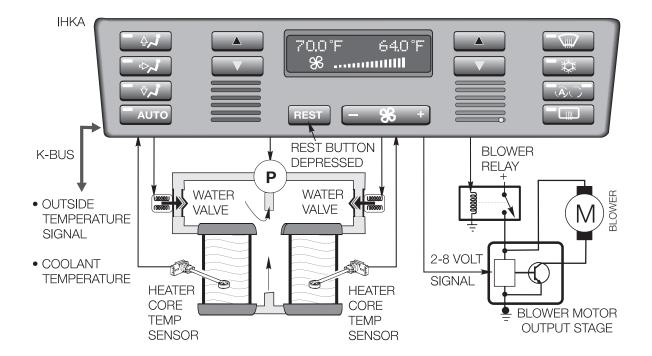
When the REST feature is activated in KL R, all of the IHKA functions are operable. This includes the blower speed, air distribution control and temperature settings.
