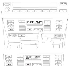
If one of the air distribution buttons is pressed when in the auto mode (1), the air distribution will come out of the automatic program, however, the automatic blower speed program will remain active and the "AUTO-symbol" will continue to be displayed in the LCD panel.
