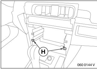
Attach speed nuts **H** to the centre console module holder.
