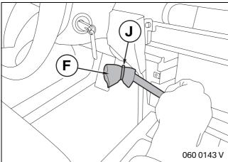
Also secure protective strip **F** using cable tie **J**.
