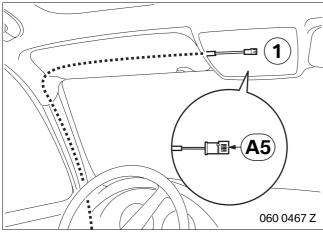
Route branch A5 to the left A pillar over the lowered headlining to the opening of the roof trim (1).
