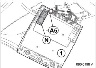
The arrow on the hands-free microphone **N** must point to the front of the car when installed.
