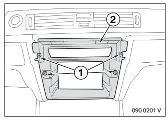
Unscrew the screws (1) on the centre console (2) module holder.
