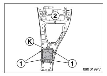
Screw controller **K** to the underside of the trim for the storage compartment (2) using the screws (1).
