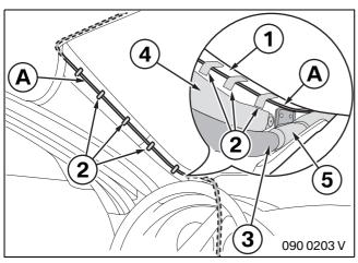
Route wiring harness **A** in the outermost corner of the A pillar (1), whilst securing with adhesive tape (2).
