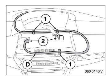
Secure LVDS cable **D** in a broad arc in the holders (1) of 8.8" on-board monitor **B**.
