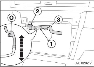
Disconnect the ventilation hose **O**. Only the last piece (1) is required. ◀
