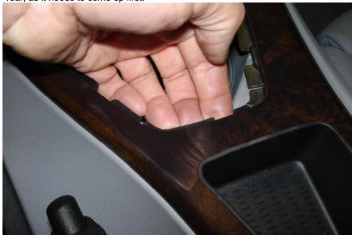
3) I used a couple old gift cards to protect the console and trim and slipped the pry bar
