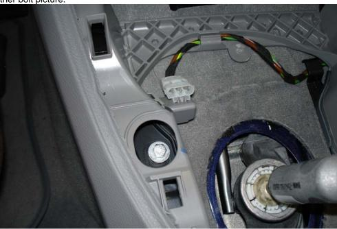
9) There are two 10mm bolts holding the back of the console on. To get the back off pull out at the top corners and then slip something like the gift card up under the lower corners to release the lock tabs. There are other DYI's that show how to do this.
