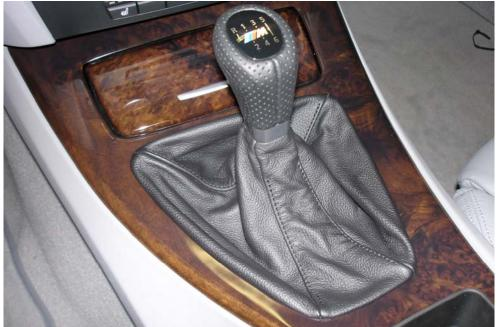
28) Side view in  $2^{nd}$  gear. These pictures show the shifter installed with the angle tipped toward the rear of the car, which matched the stock shifter.
