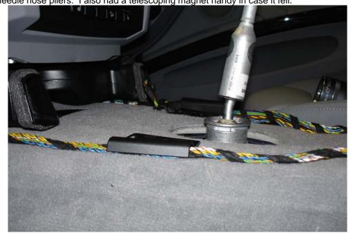
20) I didn't show it but just use 2 flat blade screwdrivers to rotate the plastic cup clockwise about 90 degrees and the shifter lifts right out. You can see the difference in the overall length is not very much. SSK on top, stock on bottom. I also wanted to show the angle of the 2 shifters. I installed the shifter angled back (top of picture) as this matched the stock shifter almost perfectly.
