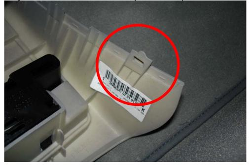
12) This connector on the left rear of the console needs to be disconnected.
