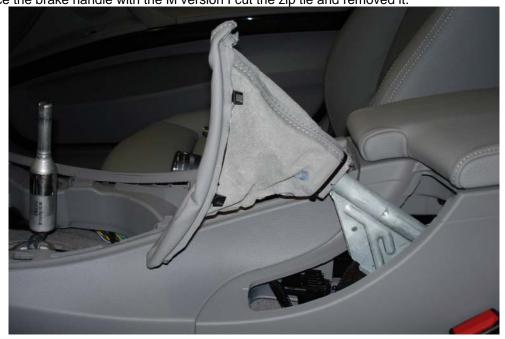
15) There is a connector under the brake lever that needs to be unclipped from the console so you can lift it off. It is easier to just slide the entire connector off than unplug anything.
