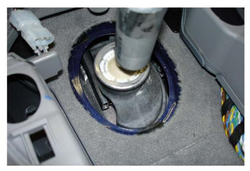
19) Just tip the back of the console up and slip it over the parking brake and now you have better access to the shifter. I was able to reach under the shifter and remover the clip with a pointed awl and needle nose pliers. I also had a telescoping magnet handy in case it fell.
