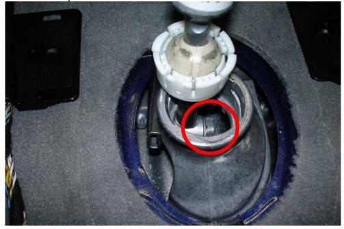
26) Just press the shifter cup back in place, install the rubber boot (using silicone spray made this very easy), reinstall the console and
