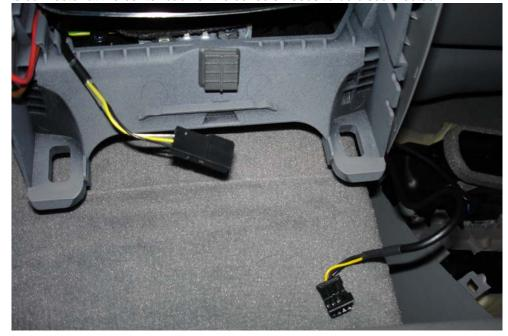
14) Pull off the cover around the parking brake lever. This comes right out. Since I was going to replace the brake handle with the M version I cut the zip tie and removed it.
