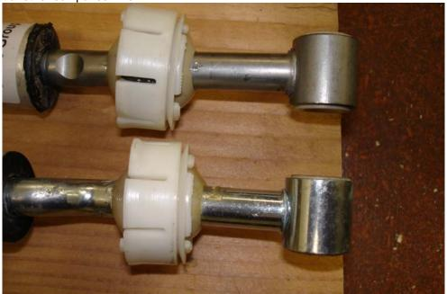
24) Here was the real trick. I installed the shifter and pivot cup and then slipped the lower pin through the shifter bushing. I tried to reinstall the clip from the bottom but found that to be very difficult. I then lifted the shifter cup back out and found I could install the clip from above very easily with a pair pf needle nose pliers. It may be possible to remove the stock shift in exactly the same way which would eliminate 90% of the method I used.
