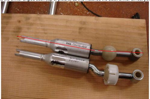
21) Difference in pivot ball to bushing hole is what makes it shift with shorter throws.
