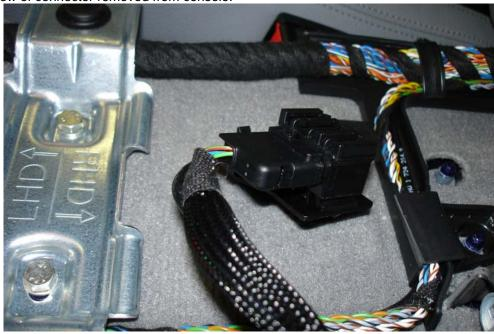
17) The connector in the front of the console just needs to slide down to come off the console.
