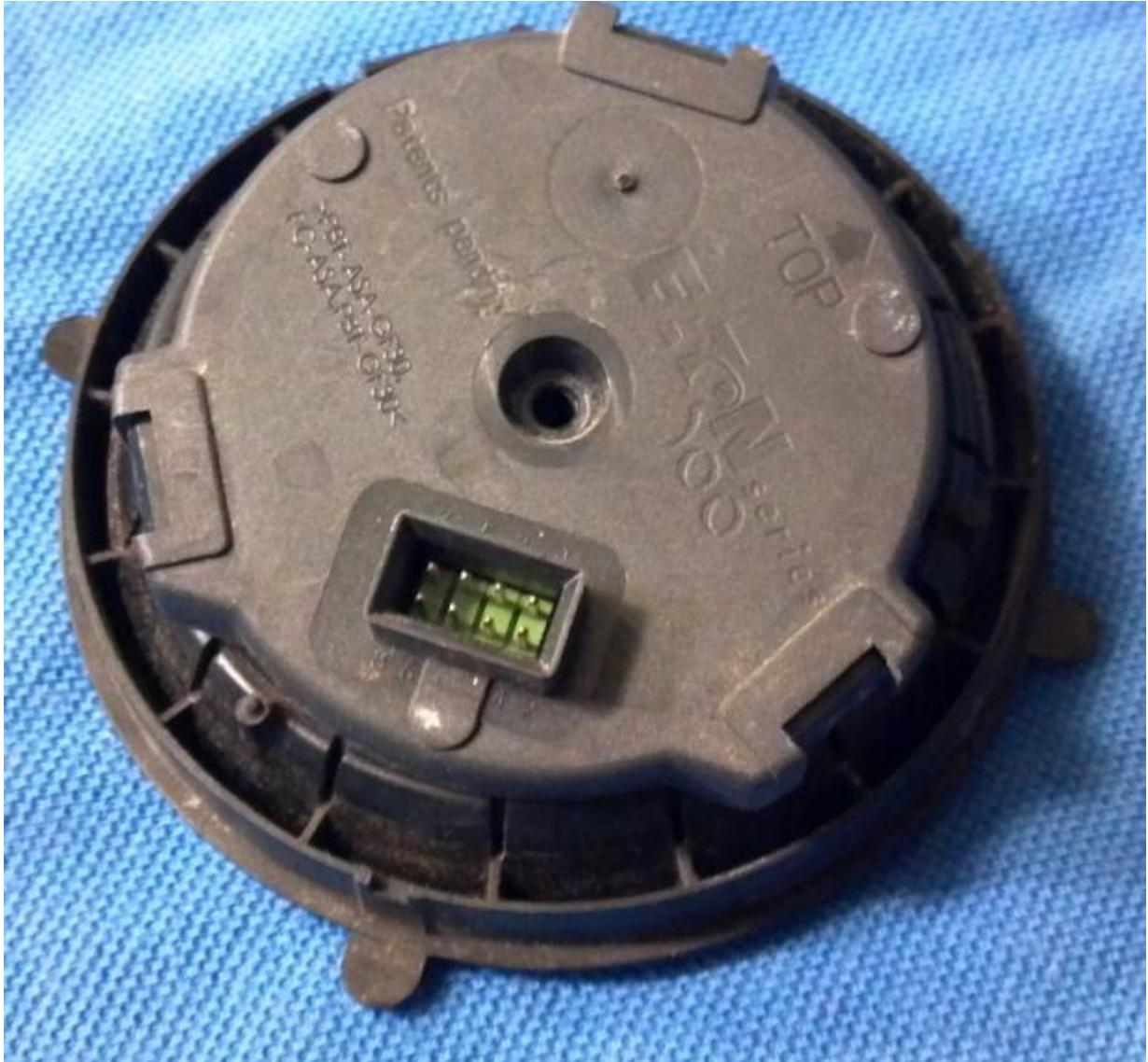
7. Not sure how to clean those little pins? Me either, so I popped the little plastic cover off the back of the motor. It pops straight off, I didn't even need any tools to get mine off. Then the pins are right there and easy to get to and clean. I used a piece of emery cloth.
