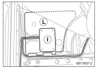
Close the USB HUB protective socket with cap  ${\bf I}$ . Insert footwell inlay  ${\bf L}$  on the floor of the car at the front left.
