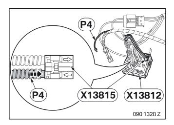
Unclip fibre optic cable casing **X13815** (SW 2-pin) from plug **X13812** (SW 16-pin) of the ASK or CCC.
