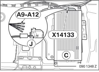
Replace the original cover cap of plug **X14133** with cover cap **J**.
