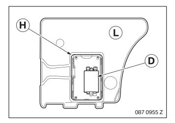
Place USB HUB protective socket **H** in footwell inlay **L**. Clip USB HUB **D** into USB-HUB protective socket **H**.
