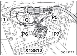
Disconnect the cables (1) from plug **X13812** (SW 16-pin) of the ASK or CCC and connect to socket casing **Q**:
