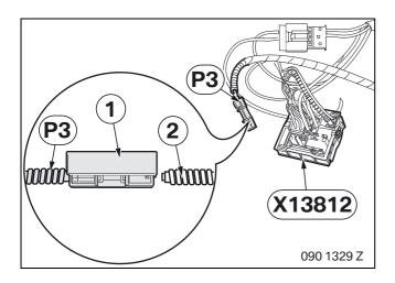
Release the fibre optic cable connector (1) of branch **P3** and connect the previously disconnected fibre optic cable (2).
