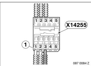
Connect the fibre optic cable (1) that you disconnected from preparation distributor station **X14280** to the cleared PIN in main distributor station **X14255**.
