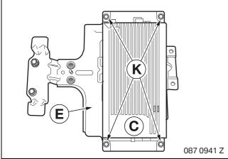
The High charger/hands-free electronic control unit is already installed in cars with SA 620 without SA 609. ◀
