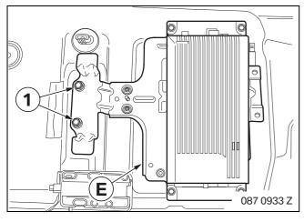
Connect holder **E** into the lugs in the car and screw on with the existing nuts (1).
