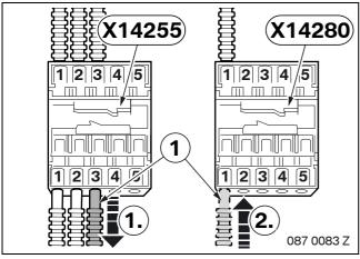
Disconnect any fibre optic cable (1) from under main distributor station **X14255** and connect it to PIN 1 of preparation distributor station **X14280**.
