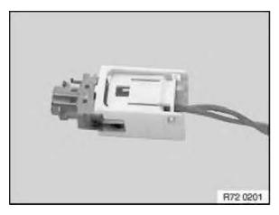
The airbag plug connection is unlocked and can now be detached from the gas generator/airbag module.
