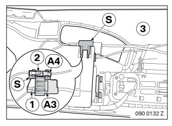
Connect branch **A3** to the plug (1) and branch **A4** to the Fakra plug (2) on the eject box.
