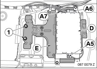
Attach the ULF holder **E** to the lugs in the car on the right-hand side and secure it with the existing nuts (1).
