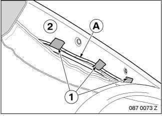
Ensure that wiring harness **A** is routed and secured behind the head airbag. ◀
