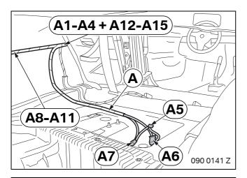
Route the wiring harness **A** from the installation site of the universal charger/electronic handsfree control module.
