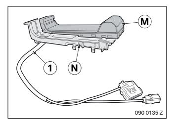
Route the cable (1) from the eject box **M** through the rear of the telephone trim **N** and clip the eject box **M** into the telephone trim **N**.
