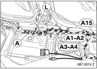
Route wiring harness **A** forwards along the standard wiring harness on the left-hand sill and secure it with cable ties **L**.
