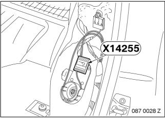
Release the main distributor station **X14255** behind the left backrest side section.
