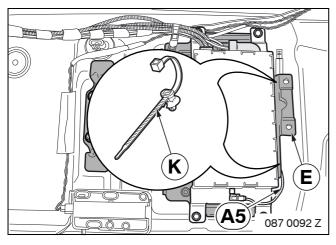
Secure the cable from branch **A5** to the side of the ULF holder **E** using a cable tie **K**.
