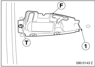
Slide in the roof aerial **F** at the front (1) and secure it at the rear with a self-tapping screw **T**.
