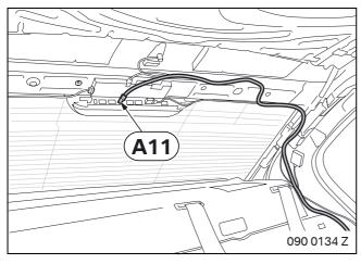
**Route** branch **A11** along the standard wiring harness to the roof aerial.
