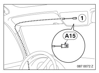
Route branch **A15** to the left A pillar through the lowered headlining to the roof trim opening (1).
