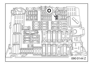
Insert fusible link O into slot 26.
