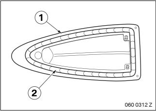
The bonding surfaces must be clean and free of grease. The temperature of the adhesive must be at least 20 °C. The hardening time of the adhesive is at least 4 hours.
