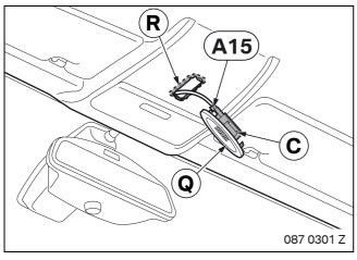
The arrow on the hands-free microphone **C** must point to the front of the car after it has been installed. •
