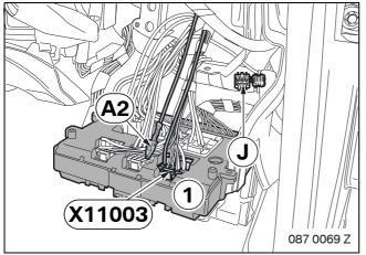
Route branch **A2** to the fuse holder behind the glove compartment (1) and connect it to PIN 6 of plug **X11003**.
