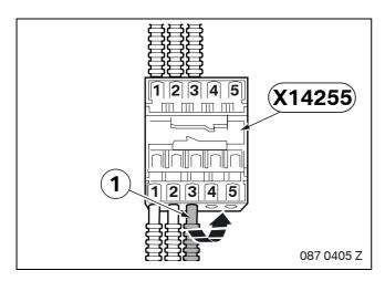
Disconnect any bottom fibre optic cable (1) from the main distributor station **X14255** and connect it to the nearest empty bottom slot.
