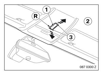
Insert the installation frame **R** from above into the opening (1) in the headlining (2) and bend the retaining lugs (3).
