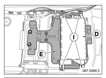
Secure the universal charger/electronic handsfree control module **D** to the stud bolt on the ULF holder **E** using hexagonal nuts **I**.
