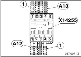
Connect branches **A12** and **A13** opposite the open fibre optic cables (1) on the main distributor station **X14255**.
