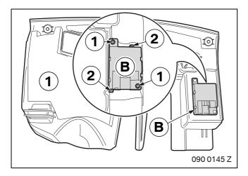
Place the Bluetooth aerial **B** on to the bolt on the pedal trim (1) until the retaining lugs (2) engage.
