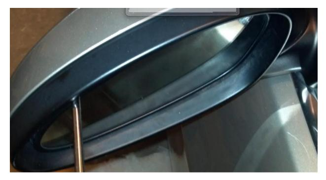
3. If your car came with heated or dimming mirrors there will be a plug on the back of the mirror glass, pop it up off the plastic backing plate of the mirror then the plug pulls right out. Make sure you are not putting any stress on either side of the wires through any of this!
