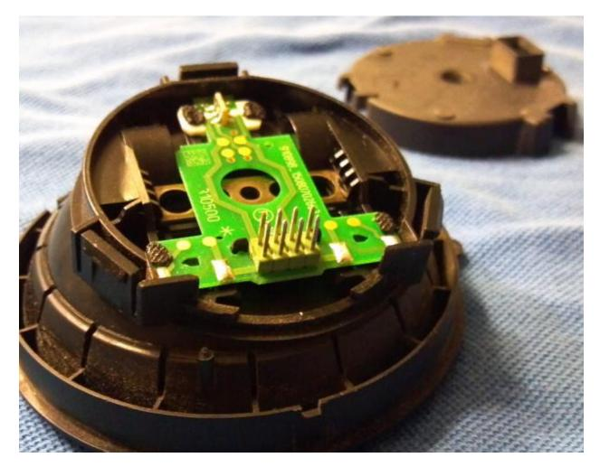
8. Now to clean the other end of the connection in the mirror housing. I used a pipe cleaner. Not sure how much this did/didn't do, but I took my time and cleaned each little hole in the connector plug just in case and blew it out with compressed air.
