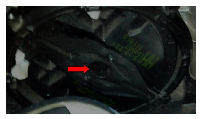
6. Now just pull the mirror motor straight out. The connection at the back of this piece is generally the cause of the problem. You need to clean this connection point.
