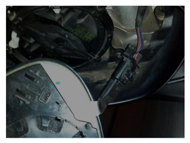
4. Lay the mirror glass out of the way in a safe place!
