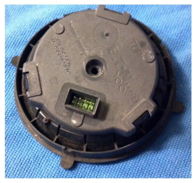
7. Not sure how to clean those little pins? Me either, so I popped the little plastic cover off the back of the motor. It pops straight off, I didn't even need any tools to get mine off. Then the pins are right there and easy to get to and clean. I used a piece of emery cloth.
