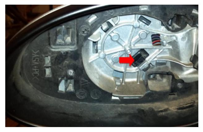
9. The TSB notes say to apply "dielectric grease" to the connectors. I don't have that/know exactly what that is. What I did have was some wire connection anti-oxidant that they sell in home improvement stores in the electrical section for a couple of bucks so I used that on both sides of the connection and I have not had any problems with mine yet...
