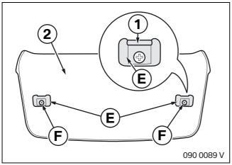
The retaining edge (1) of the bracket for the roller sun blind **E** must be aligned with the auxiliary brake light cover (2) as illustrated. •
