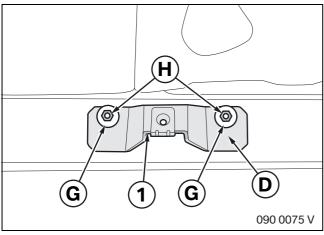
Fit bracket for rear window shelf **D** onto the screws on the underside of the rear window shelf with recess (1) facing towards the rear. Lightly secure roller sun blind **A** with washers **G** and nuts **H**.
