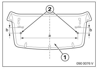
Mark dimension a centred on the inside of the cover for the auxiliary brake light (1).
