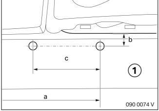
With the aid of dimensions a, b and c, drill  $\emptyset$  4.2 mm holes in the rear window shelf (1).
