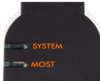
Fig. 12 Light-emitting diodes on the ICOM B housing
