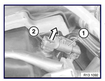
Unlock and disconnect the connector (1). Remove charging pressure sensor (2) in direction of arrow.
