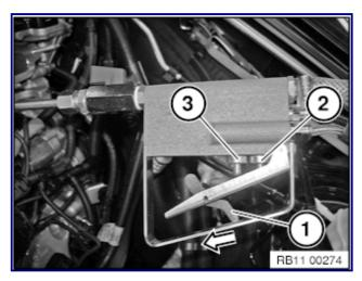
Slide locking lever (1) to the front in direction of arrow.
