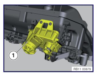
Remove swirl-flap actuator (1) from intake plenum.
