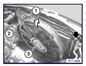
Unlock and disconnect the connector (1). Release screw.
