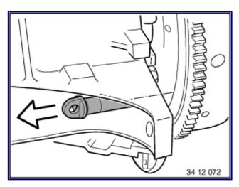
Remove protective cap in direction of arrow.
