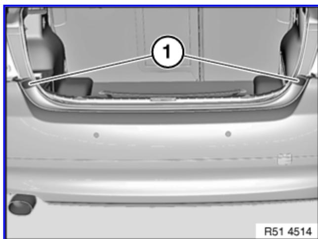
Lever out cover (1) and release screw underneath.
