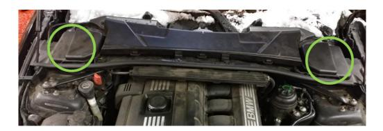
Remove rain sensors from cowling. (Twist and pull from retainers)
