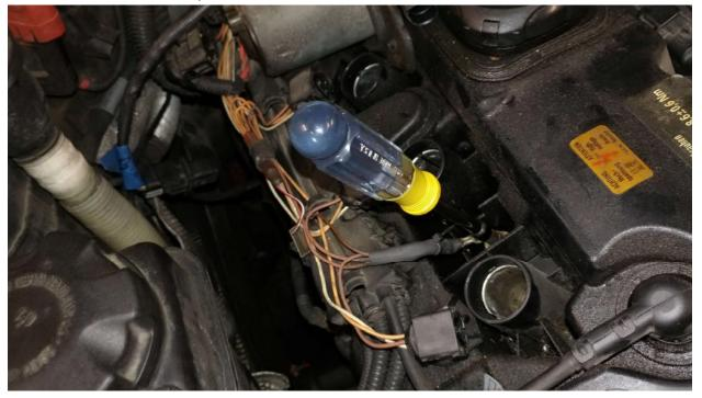
• Disconnect valvetronic servo motor from injector loom
