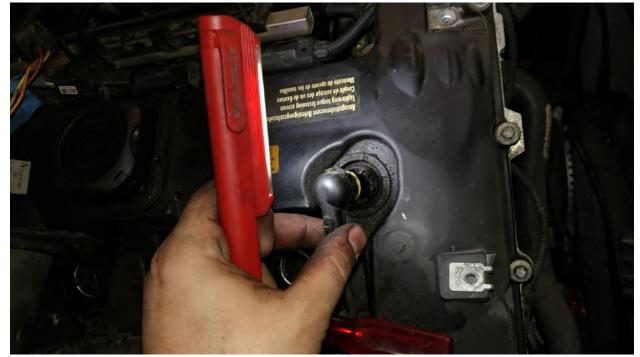
• Remove 6x injector plugs from loom (pry tabs away from plugs and pull away)
