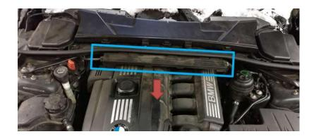
• Remove large wire loom from cowling assembly. (pry open with thin and small flat bladed screwdriver
