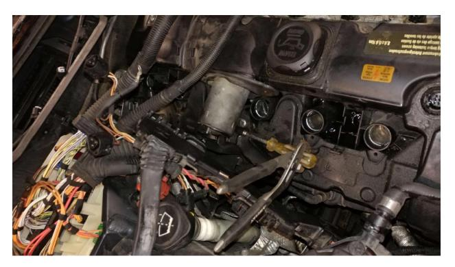
• Remove bolt under valvetronic servo (10mm socket)
