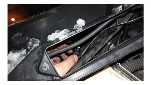
• Disconnect and remove upper shock tower braces (2x E12 bolt (dark blue circle) and 1x E14 bolt(dark green circle))
