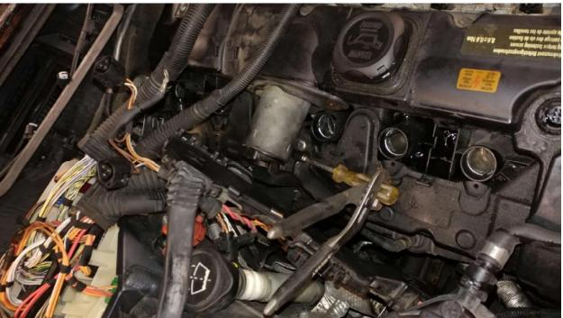
• Remove valvetronic servo, insert 4mm allen wrench into end of servo motor, rotate clockwise until resistance is felt, then pull servo horizontally outwards.
