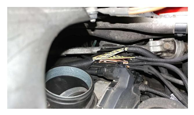
• Remove vacuum lines from manifold (3x vacuum lines -- 2 are pictured one is underneath intake manifold -- press on sides of connector and pull away) (1x vacuum line has electrical connector - disconnect by lifting tab and pulling wire away as shown).
