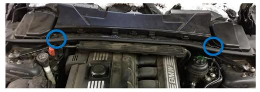
• Remove over-engine wire loom by pulling forward separate covers and separate wires
