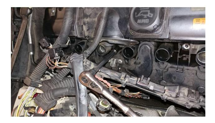
• Remove position sensor relay connection wire from top of valve cover (pry tabs on sides outwards and lift up)
