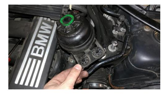
Remove intake snorkel (torx bit and clips)
