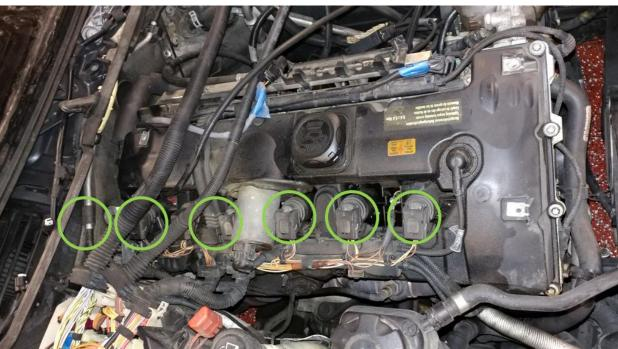
Remove coil plug tubes (6 pcs) using snap ring pliers
