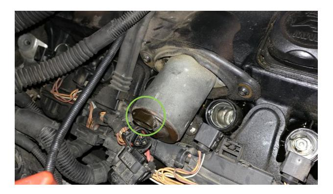
Remove valvetronic servo bolts (2x E8 on flange and 1x on bottom)
