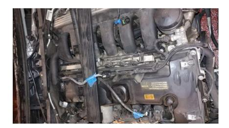
• Disconnect temp sensor near oil filter housing, (compress lock tab and pull away from base of sensor)
