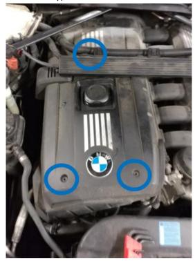
Remove vacuum accumulator hold down bolts (2x 10mm hex nuts)
