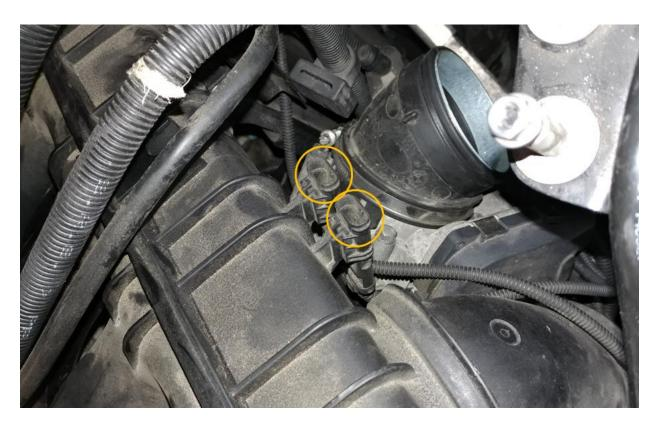
• Remove high pressure fuel line stay from intake manifold (1x T25 bit screw -- aft side of intake manifold)
