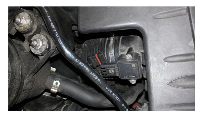
• Remove elbow and Helmholtz resonator; 1x 5mm bolt on strap
