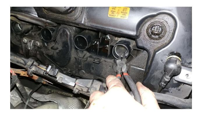
• Disconnect ground nuts on injector harness (2x 5/16" nuts? (metric sizes didn't fit well) one at front and one at back). Remove standoffs underneath nuts.
