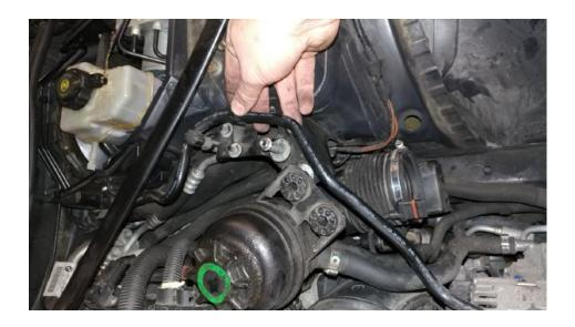
• Remove cowling, disconnect windshield washer wires
