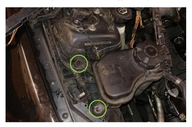
Remove valve cover bolts (E10 bolts)
