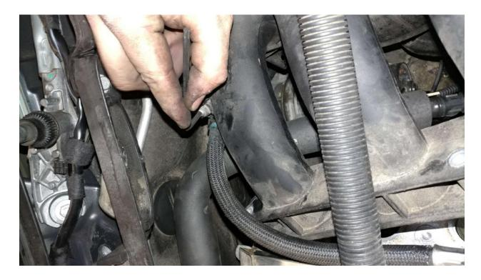
Manipulate intake manifold and remove it from vehicle, engine should appear as shown (note:
