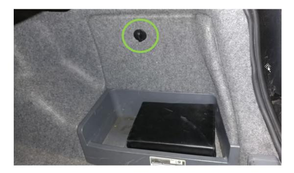
• Disconnect both terminals of the battery 10mm mm on (-) terminal strap (red circle), 13 mm on positive relay (blue circle underneath flip up cap)
