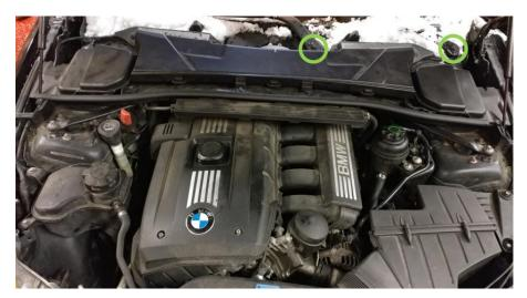
Remove electrical box cover and brake fluid covers
