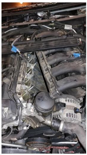
• Separate lower wire loom from intake manifold (un-clip and move out of way) -- Remove all connected electrical wiring as well taking care to ensure proper and safe removal of each connector
