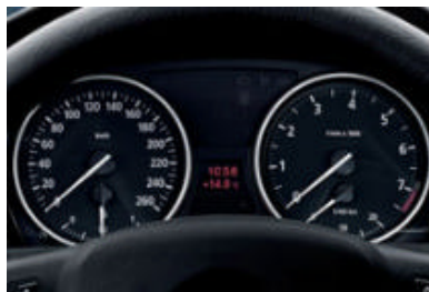
■ Instrument panel with analogue indicators and red backlighting, speedometer with integrated fuel level display, rev counter with fuel consumption display, LC display for total and trip mileage counter, outside temperature display and clock.
