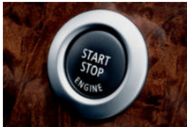
■ Start/Stop button for starting the engine. After inserting your ignition key, you can start and stop the engine by pressing this button.
