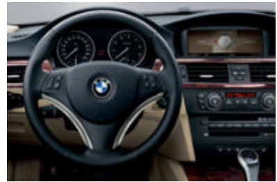
□ Leather sports steering wheel (369 mm diameter), three spokes, incl. gearshift lever handle and steering wheel with chrome trim and handbrake lever handle finished in leather, multifunction buttons for remote control of radio/telephone (both optional); also available without multifunction buttons.
