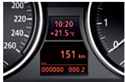
■ On-board computer displays information about average speed, average fuel consumption and range.
