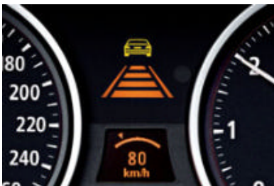
□ Active Cruise Control enables comfortable driving at a pre-selected speed. When driving in columns of traffic, your BMW automatically adapts to the speed of the preceding vehicle and maintains a preset distance. (Only available for six-cylinder models.)
