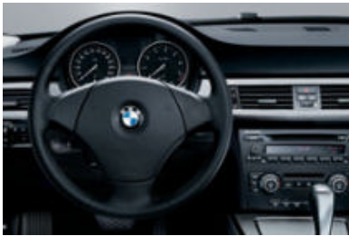
■ Standard steering wheel (375 mm diameter), three spokes.
