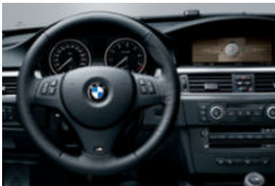
□ M leather steering wheel: Provides excellent grip due to its thicker rim. The integrated (optional) multifunction buttons can be used to operate the radio, CD player and telephone (if present).
