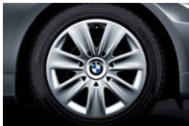
■ Steel wheels with full wheel covers , 7 J x 16", 205/55 R 16 tyres (standard on 318i, 320i and 318d).
