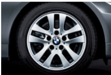
□ BMW light-alloy wheels double-spoke styling 156, 7 J x 16", 205/55 R 16 tyres (standard on 325i and 320d).
