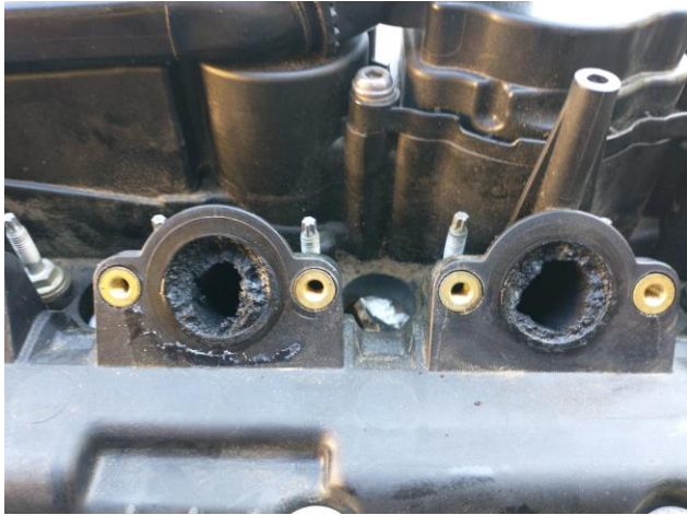
Left – caking inside intake runners in rocker cover. Right – yes, there is a valve in this photo!
