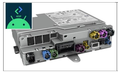
The HU-H6 was introduced in the U11 in late 2023. In BMW vehicles from 2023 onwards, the control interface of the **HU-H6** will be operated via touch functions or voice control. The familiar I-Drive controller has been removed.
