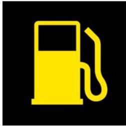
The fuel reserve level is not indicated by an indicator lamp as in the previous models. A fuel pump symbol lights up for 23 seconds in the liquid crystal display as soon as the reserve level is reached (2.1 gallons).
