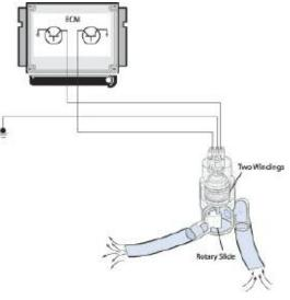
The Idle Air Actuator is controlled by the ECM modulating the ground signals (PWM at 100 Hz) to the valve. By varying the duty cycle applied to the windings, the valve can be progressively opened, or held steady to maintain the idle speed.
