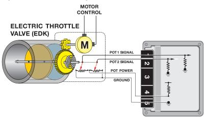
**Total Intake Air Flow Control** is performed by the ECM simultaneously operating the EDK throttle control and the Idle Air Actuator.
