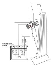
The Accelerator Pedal Position is monitored by the ECM
