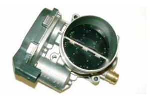
This integrated electronic throttle reduces extra control modules, wiring, and sensors. Adjusting electronic throttles is not permitted, the throttle assembly must be replaced as a unit. The adaptation values must be cleared and adaptation procedure must be performed using ISTA.
