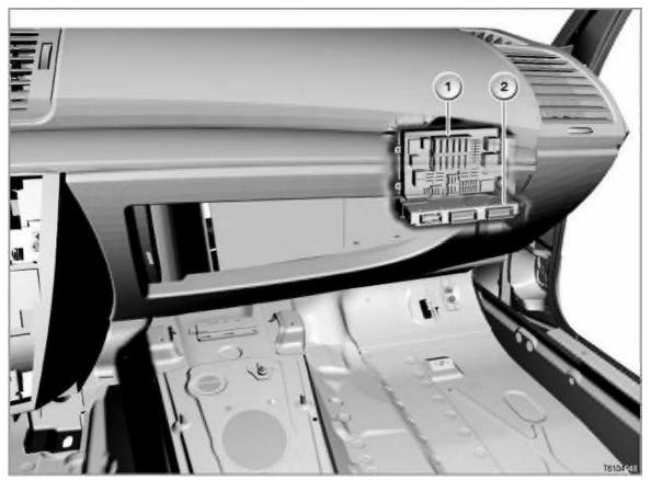
The illustration shows the example of the junction box installation location on the E87.
