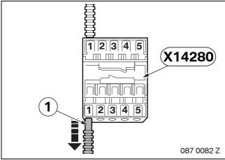
Disconnect the bottom fibre optic cable (1) from PIN 1 on preparation distributor station **X14280**.
