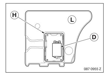
Place USB HUB protective socket **H** in footwell inlay **L**. Clip USB HUB **D** into USB-HUB protective socket **H**.
