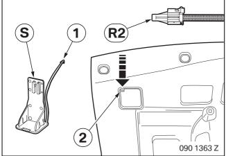
Secure the Flash adapter cover **S** using securing strap (1) from the outside to the pedal trim (2).
