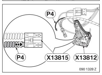
Disconnect the cables (1) from plug **X13812** (SW 16-pin) of the M-ASK or CCC and connect to socket casing **Q**:
