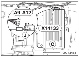
Replace the original cover cap of plug  $\bf X14133$  with cover cap  $\bf J$  .
