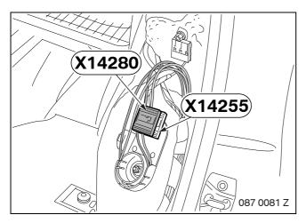
Release preparation distributor station **X14280** and main distributor station **X14255** behind the left backrest part.
