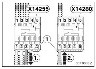
Disconnect bottom fibre optic cable (1) from main distributor station **X14255** and connect it to PIN 1 of preparation distributor station **X14280**.
