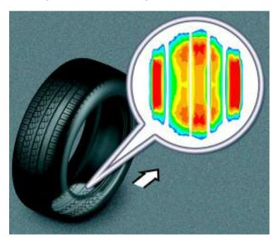
The tire contact patch therefore describes the area of road which is touched by the tire when the vehicle is in operation.
