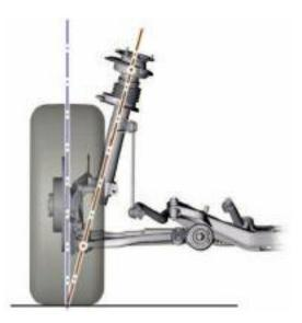
Pivot Axis (shown here using the single-pivot spring strut front suspension)
