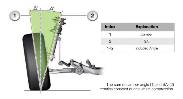
Depending on the type of alignment equipment used, SAI and IA can be measured by raising the vehicle. Look for any excessive deviations from side to side. This could indicate possible chassis (frame) damage or bent components (strut/spindle).
