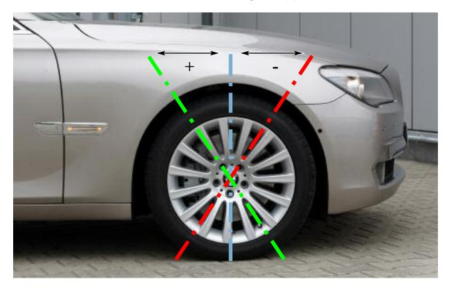
Most vehicles have a caster angle from zero degrees to a positive angle. Negative caster is not very desirable because it reduces the vehicle stability especially at high speeds. BMW vehicle always have a positive caster angle. Positive caster promotes high speed stability and provides feedback to the driver.
