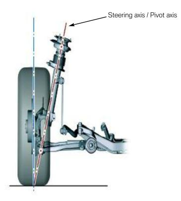
Wheel suspension kinematics can cause this axis to move when the steering angle changes.
