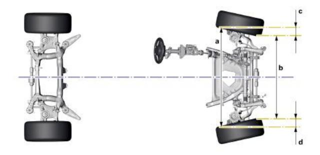
Toe has a major influence on vehicle handling, straight line stability and the position of the steering wheel. An incorrect toe setting will have a negative effect on tire wear. A toe angle which is out of specification will cause the tires to wear in a relatively short time.
