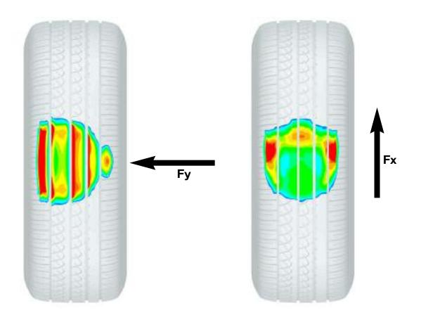
Tire contact patch affected by lateral force, e.g. cornering (Fy) Tire contact patch affected by logitudinal force, e.g. braking force (Fx)
