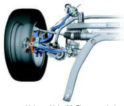
Universal joint McPherson axle / Determining the lower pivot point
