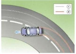
**Oversteer:** Vehicle slides outwards via the rear axle
