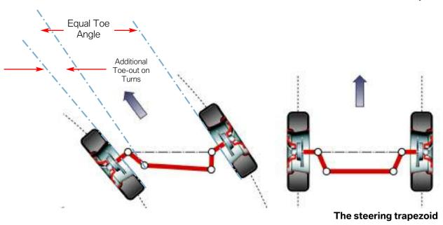
If set correctly, the toe-differential angle will be the same for both left and right-hand steering inputs, taking into account permissible angular tolerances. The resulting angular difference (toe differential angle) between the angles of the steering arms increases as the steering angle increases.
