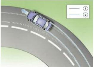
Understeer: Vehicle slides outwards via the front axle
