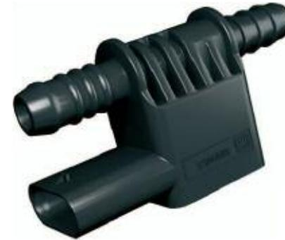
The integrated fuel temperature sensor is identical to the fuel temperature sensor used in the E90. The fuel pressure sensor is also integrated in the housing. Both the fuel pressure sensor and the fuel temperature sensor features two separate connections in a common connector housing that has four pins.
