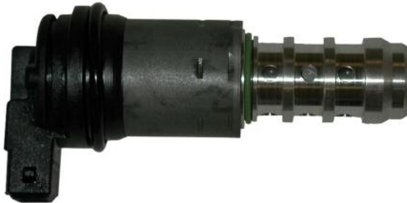
The variable camshaft control serves the purpose of increasing torque in the lower and medium engine speed ranges. The VANOS solenoid valve activates the VANOS adjustment unit on the intake side. The VANOS solenoid valves are driven by the ECM control unit.
