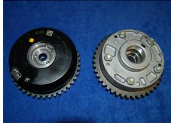
The VANOS units on the N63 engine differ from the VANOS units on the N62 engine. The function is identical but some components have been omitted and the VANOS unit has been optimized.
