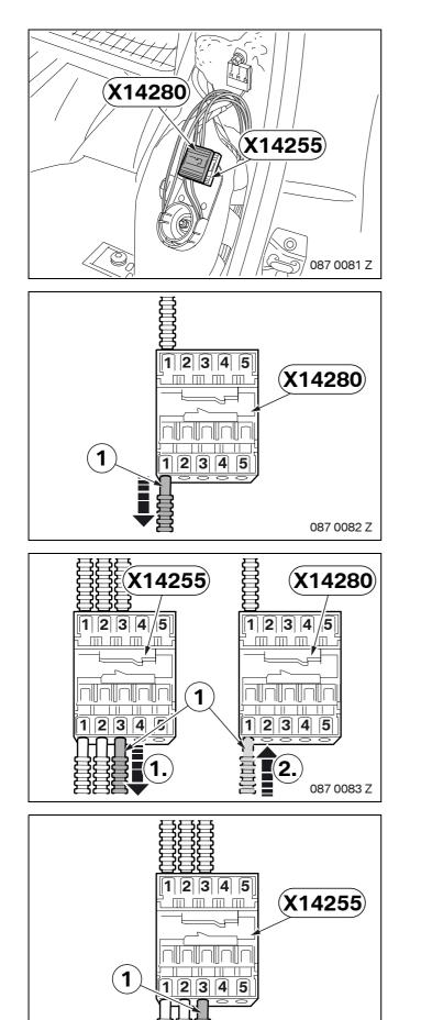
Release the preparation distributor station **X14280** and the main distributor station **X14255** behind the left backrest part.
