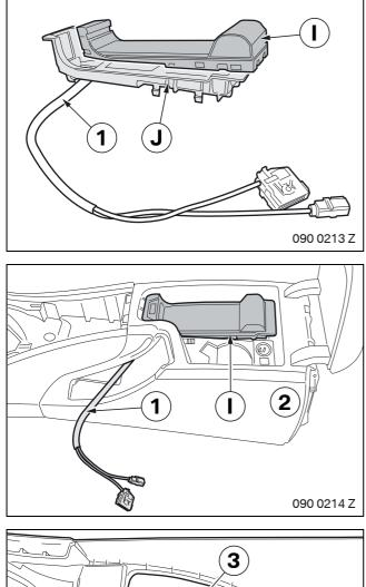
3 2 3 1 X4545 090 0215 Z Route the cable (1) from the eject box I through the rear of the telephone trim **J** and clip the eject box I into the telephone trim **J**.
