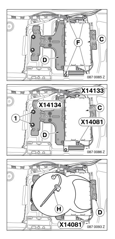
Secure the universal charger/electronic handsfree control module **C** to the stud bolt on the ULF holder **D** using hexagonal nuts **F**.
