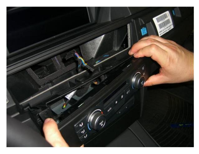
3. Remove cover plate from Multimedia unit keypad. Like all the other parts it is just snapped in place.
