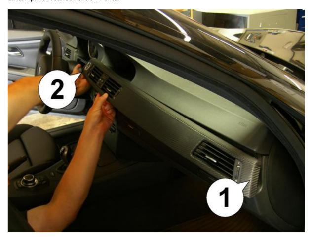
2. Pull out the Climate Control panel and disconnect the plugs on it's back.
