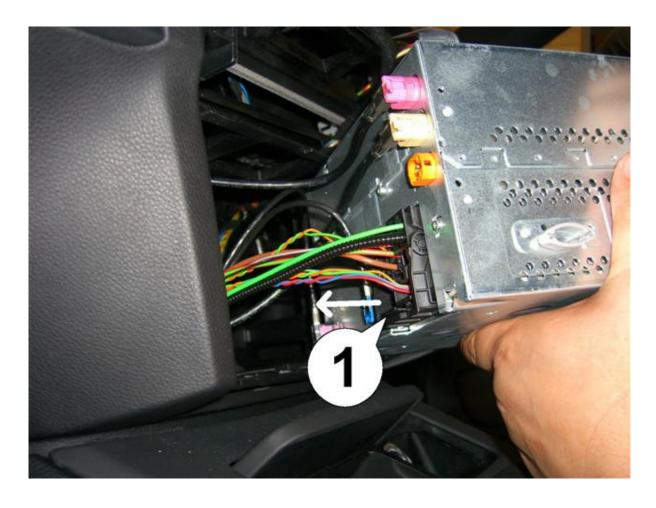
Disconnect CIC unit. Find spitted CAN wires – pins 9 and 10. Cut these wires. Connect emulator like in picture
