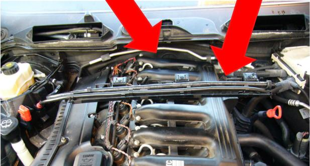
10. Lift away the inlet manifold – be wary of the vacuum pipe from the EGR valve, personally I could not remove this, in which case the manifold can be rotated and rested on the fan housing (seen here bottom left).
