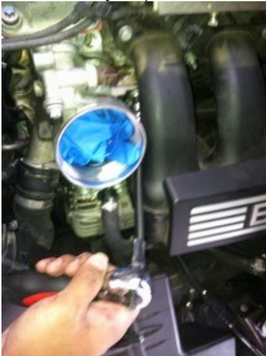
2d. With an 8mm wrench, unbolt the easiest bolt. [Notice the aluminum, I covered the alternator so that oil or coolant doesn't ruin it. I also wrapped the brown oil pressure switch with tape just in case.
