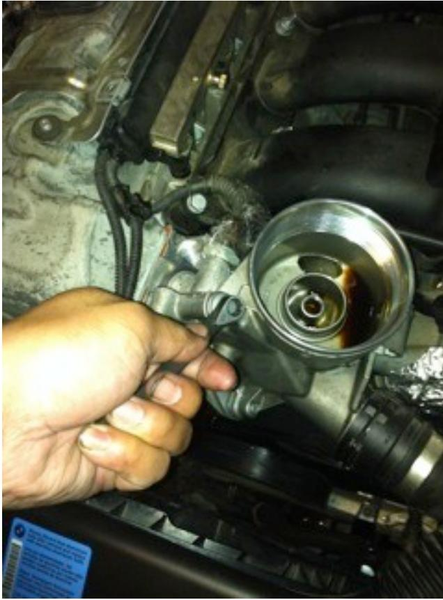
4a. Once all bolts are removed, you can slowly separate the housing from its base port. Slowly remove old gasket with a pick to get it all out in one piece.
