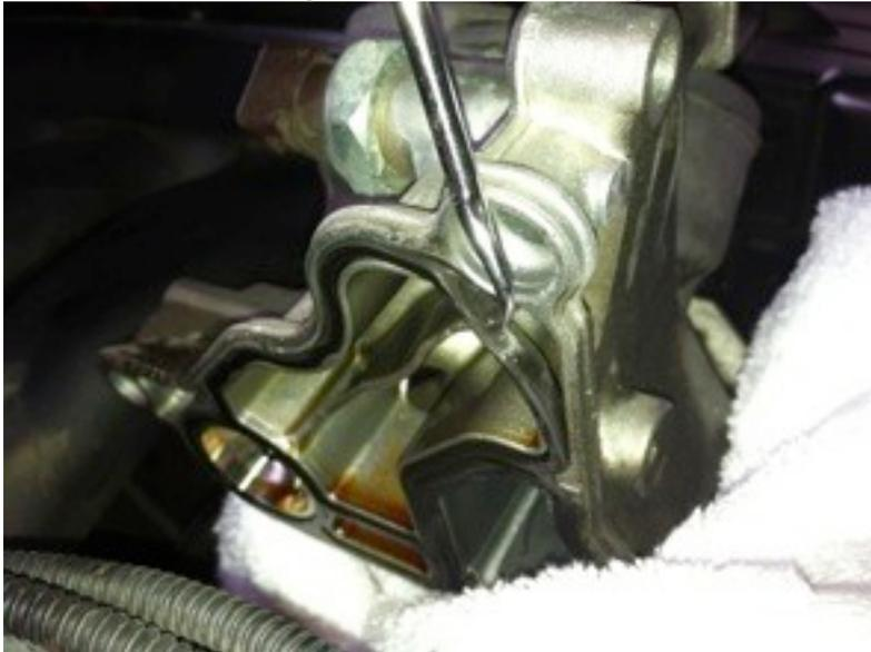
4b. Use brake cleaner to clean surface and contact surface on both sides. I didn't take a picture cleaning it but I do have picture of what you do need to clean. The **red arrows** shows the residual gasket that is stuck on the base. Be careful when cleaning this surface, do not scratch it with a screw driver. I mainly used brake cleaner, chrome
