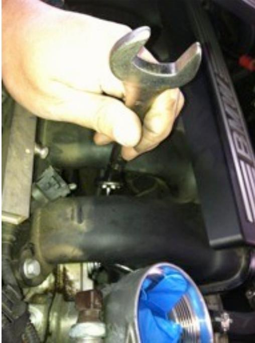
2c. Once loosened, I used a flexible 8 in. 3/8 extension with an 8mm bit to thread the whole bolt out. [Blue plastic in the housing is a nitrile glove I used to cover the port
