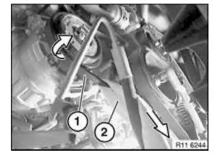
Rotate engine with special tool 11 6 480 in direction of engine rotation.
