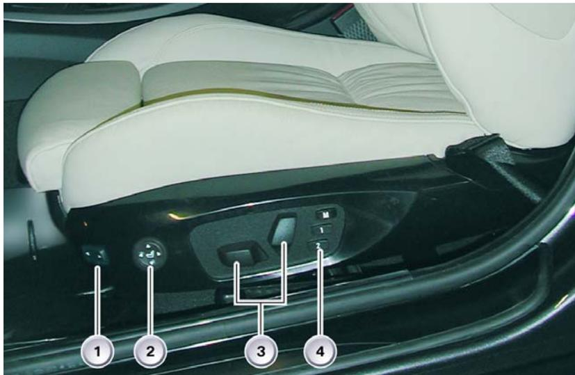
**Lumbar support button, seat adjustment switch and memory buttons**
