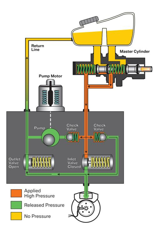
Typical ABS/DSC Hydraulic Schematic
