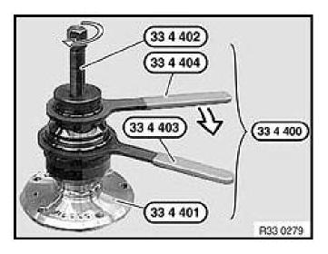
Rear Wheel Bearing Race-Removing Kit 83 30 0 493 416
