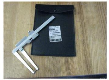
Veiner caliper for measuring brake disc 88 88 6 341 280 (34 1 280)
