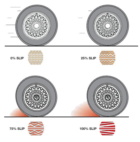
The transmission of braking forces and the retention of Lateral Locating Forces are inverse. That is to say as braking forces increase the locating forces decrease.
