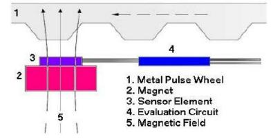
The sensor element converts the changes in resistance into voltages. The small amount of voltage coming from the sensor element (1 to 100mV) is monitored by the evaluation module.
