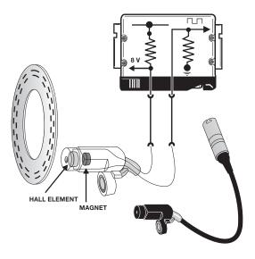
This creates a DC square wave signal with a low of .75 volts and a high of 2.5 volts.
