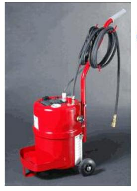
BMW recommends pressure bleeding with the "Power Probe Bleeder", which utilizes a variable electric pump set at 2 bar (30psi). Proper bleeding of current BMW vehicles will also require the execution of the brake bleeding service function via the tester.
