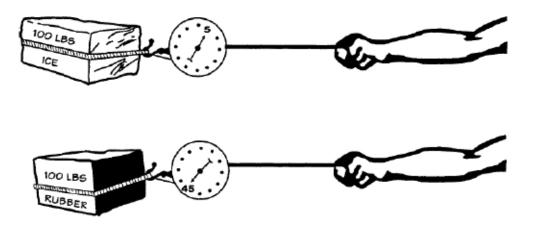
The above example illustrates how the type of friction surface and the material can influence the coefficient of friction (COF).
