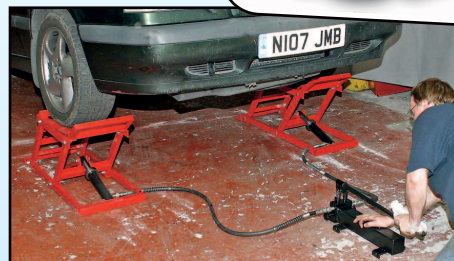
Drive or push the car up them, and pump the ramps to full height.
