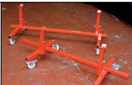
These stands are fully mobile, and both the supports' height and distance apart are adjustable.
