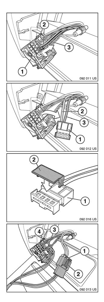
13. Remove the following wires (2 & 3) from connector housing (1):
