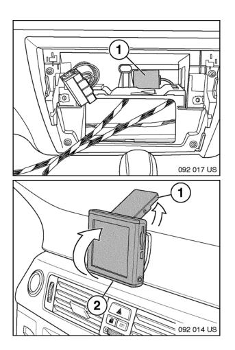
17. Secure power converter box (1) behind dash bracing in radio cavity.
