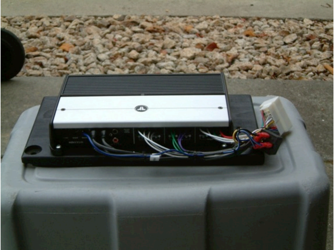
JL XD 600/6 mounted to the Amp Mount Board with Technic Harness
