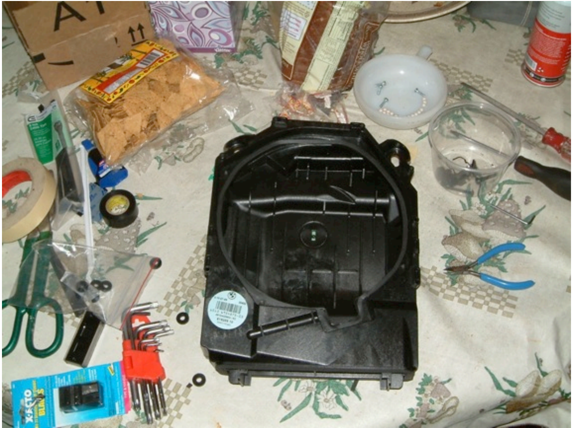
Under Seat Speaker Housing with Foam Seal applied
