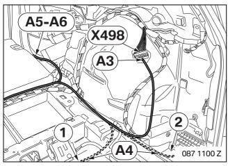
Before installing amplifier **C** set switch (1) to position 1. Remove protective film from adhesive strips (2).
